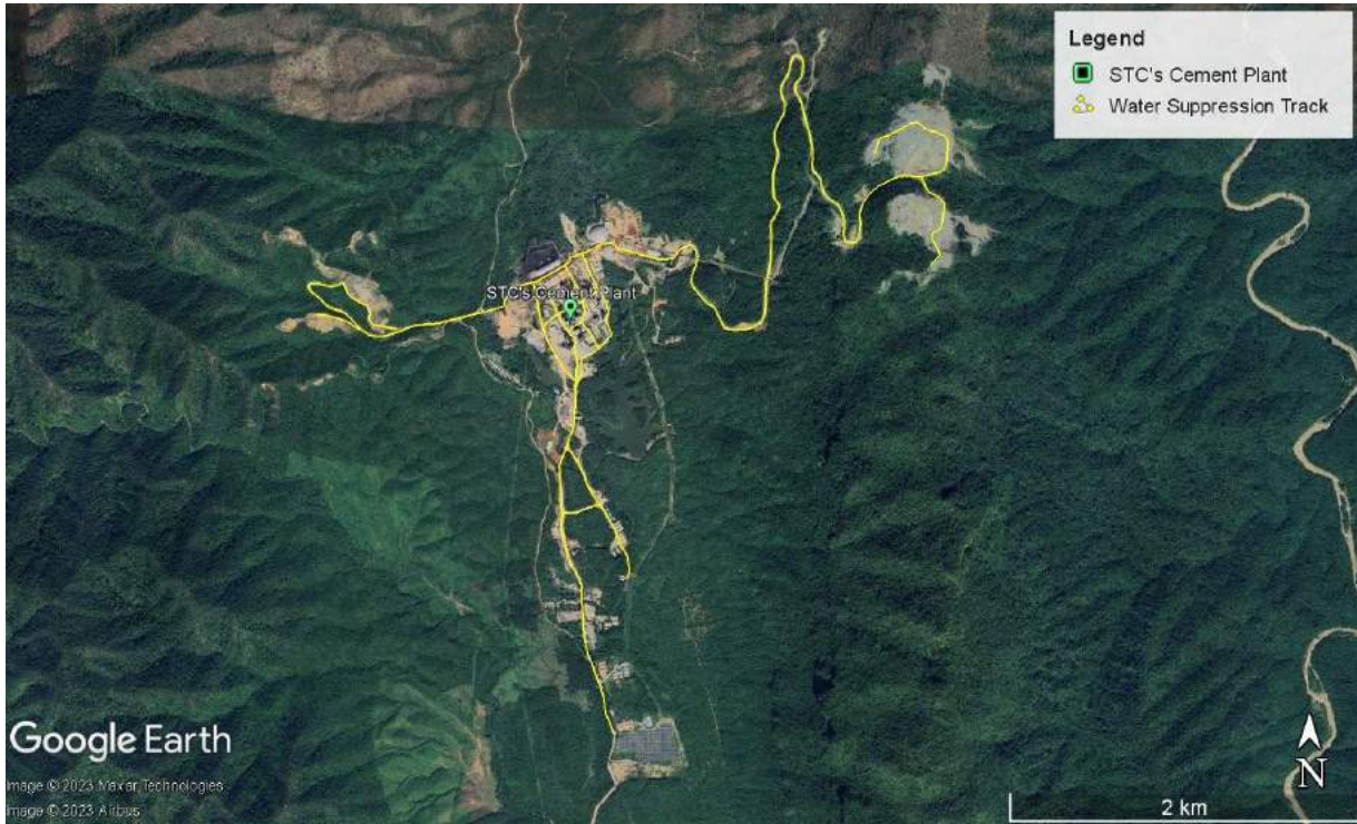
Figure- Water Suppression Map to mitigate dust emission in plant site
